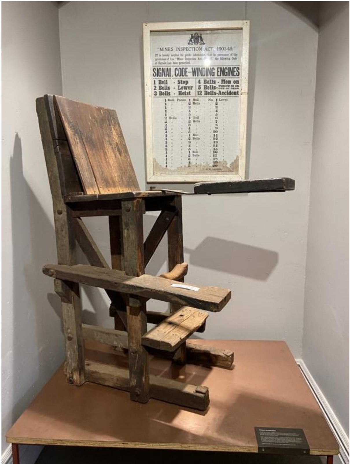
Signalman's Chair and Winding Engine Signal Code Cobar Mining Museum [photograph by research team]
